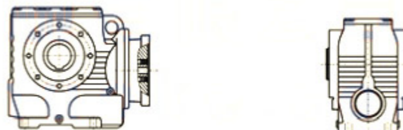
SA(S, SF, SAF, SAZ) ...Y... 电机用户自配或配特殊电机时需加联接法兰 When equipping the user's motor or the special one, the flange is required to be connected
